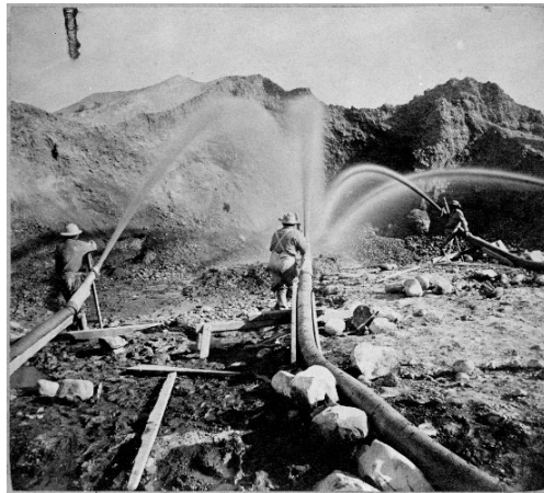
Hydraulic mining near French Corral, Nevada County, CA, 1860-1870. Courtesy of the Library of Congress.
